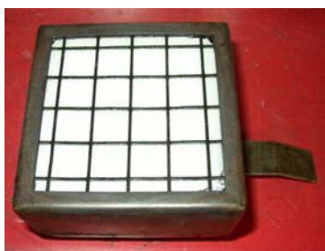
Figure 3-3: ASTM E1354 Cone calorimeter sample holder
